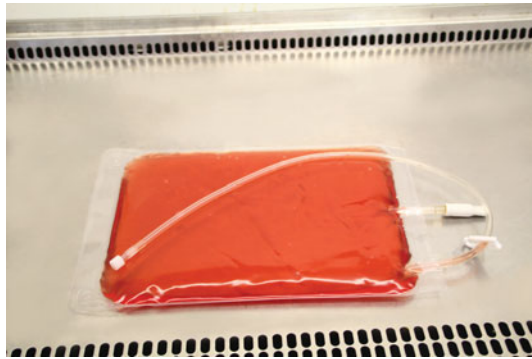
Figure 1. Corning gas-permeable cell culture bags are equipped with a septum port (up) and tubing with a female Luer lock and cap (down).
