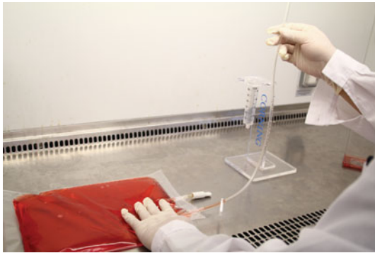
Figure 5. Remove as much excess air from the Corning cell culture bag as possible.
