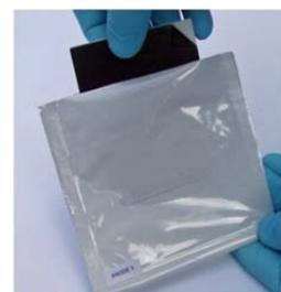
1.4. Open Lightning Blot **Envelope 2** using scissors to cut between the two tabs and place the assembly on top of the Anode 1 with the dark blue cover sheet on top. Use the folded corner tab (see arrow) to simplify removal of the cover sheet from the PVDF membrane. This corner (see ★ on Figure 3) can be used to mark the membrane using a pencil for identification.
